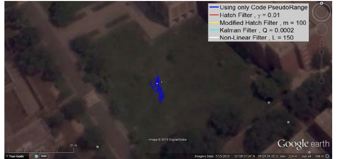
Figure 9. Position computation using real GPS data after smoothing pseudoranges from each algorithm
