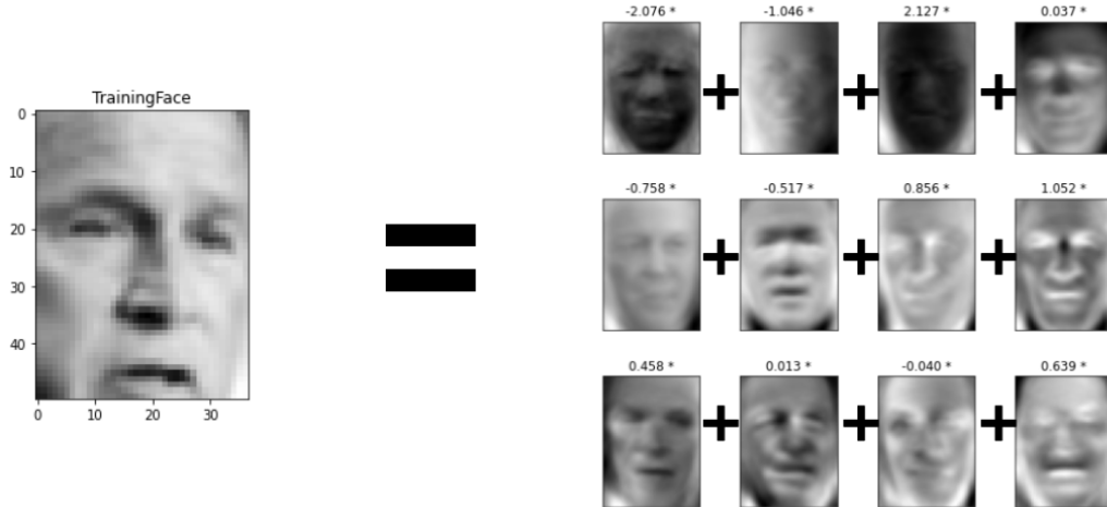
Figure 15: Represent a face as a linear combination of top k eigenfaces
