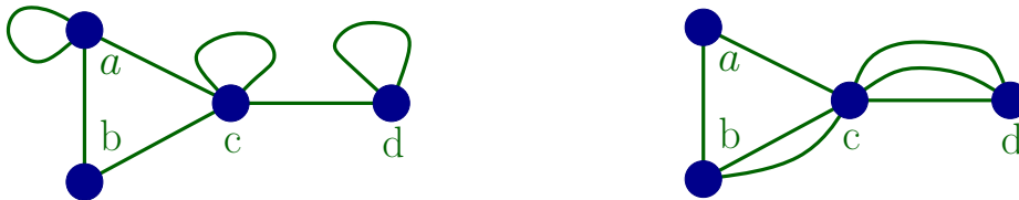
Figure 16: A graph G = (V, E) , where V is the vertex set, is a pseudograph if E is a set of edges where G is a multigraph if E is a multi-set of edges i.e. there may be multiple edges between a pair of nodes. Both types of graphs may have self loops on nodes.
