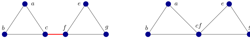
Figure 19: The min cut in G is not necessarily at least as large as the min cut in G \setminus \{u, v\} . The min-cut in the graph on the left is [\{a, b, c\}, \{e, f, g\}] is of size one, whereas there is no cut of size one in the graph after contracting edge (c, f) on the right.
