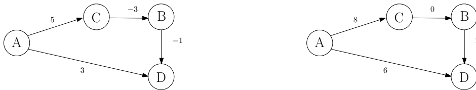
Figure 17: In the graph on the left, d(A, D) = 1 via the path ACBD . The largest absolute value edge weight is 3. We add 3 to all the weights. In the resulting graph, on the right, AD is the shortest path from A to D with length 6.
