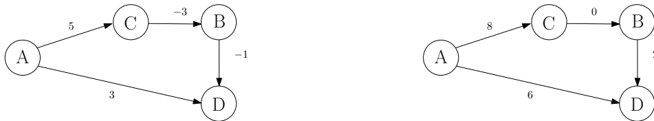
Figure 20: In the graph on the left, d(A, D) = 1 via the path ACBD . The largest absolute value edge weight is 3. We add 3 to all the weights. In the resulting graph, on the right, AD is the shortest path from A to D with length 6.
