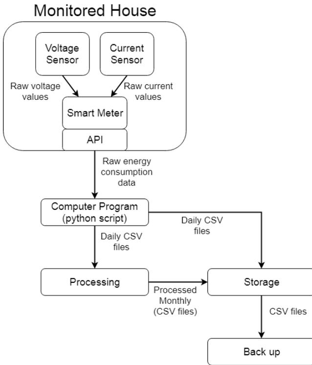
Figure 5: Data flow diagram for data collection architecture
