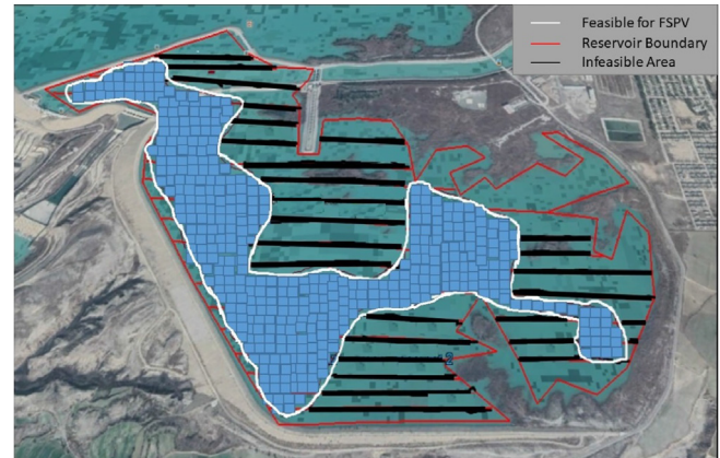
Fig. 9. Feasible (Blue area) and Infeasible (black lines) areas of Reservoir 2 of Ghazi Barotha. (For interpretation of the references to colour in this figure legend, the reader is referred to the Web version of this article.)
