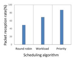
Figure 5. Multihop packet reception rates with different energy scheduling algorithms.
