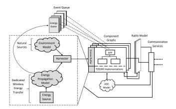
Figure 1. Extending TOSSIM architecture [11] for modeling intermittently powered embedded networks (grey): extensions include *energy source* and *harvester* components for modeling respective phenomena, wireless *energy propagation* model, and a new event type for registering energy transfer operation into simulation.
