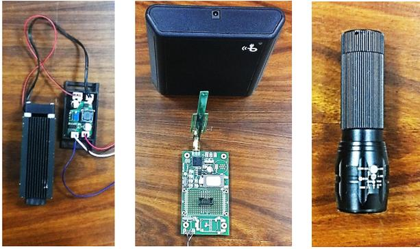
(a) Laser module (0.8W) (b) PowerCast RF module (3W) (c) Cree LED torch (3W)
