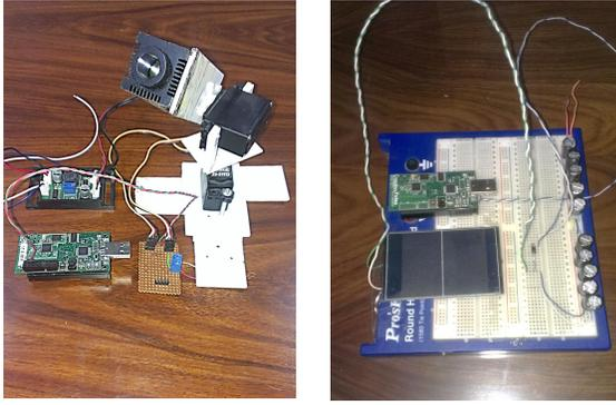
(a) LAMP master: TelosB with  $\mu$ -power beaming and pan-tilt (b) LAMP leaf: TelosB with monocrystalline solar panel
