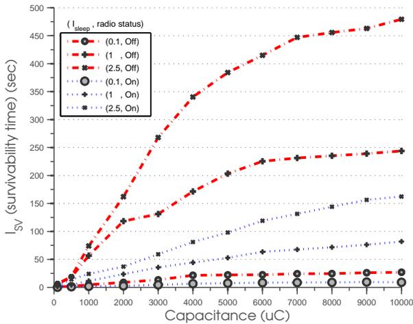
Fig. 10.  $I_{SV}$  as a function of  $I_{sleep}$  (for recharging), and capacitance (charge capacity).
