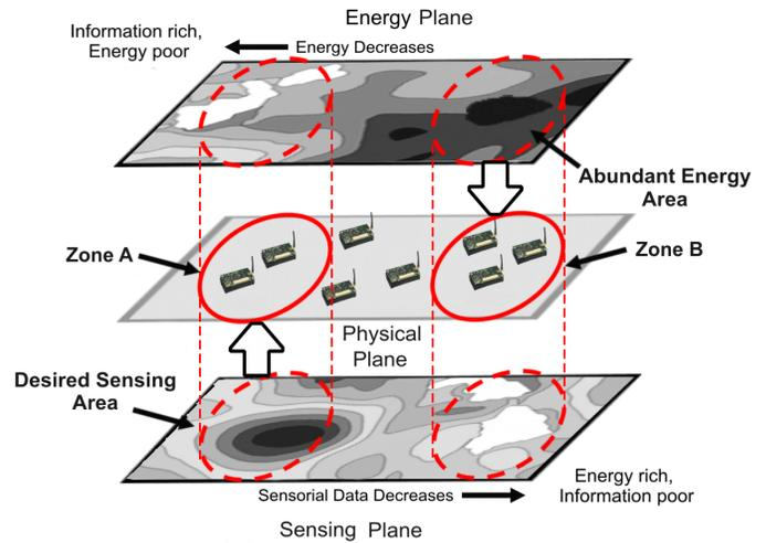
Fig. 2. Decoupled energy and sensing planes in WSN. These planes are spatially uncorrelated in most deployments.
