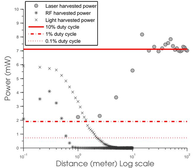
Fig. 4. Harvested power at different ranges (log scale). Also shown are power requirement for TelosB operation at different duty-cycles.
