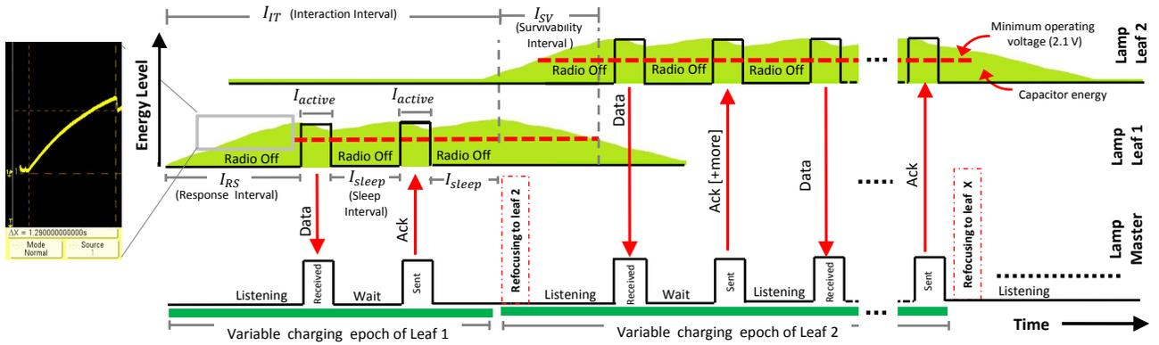
Fig. 7. LAMP Control Protocol: A master focuses laser on a leaf for a charging epoch in which leaf duty cycles to exchange control information; master then refocuses based on a scheduling policy.
