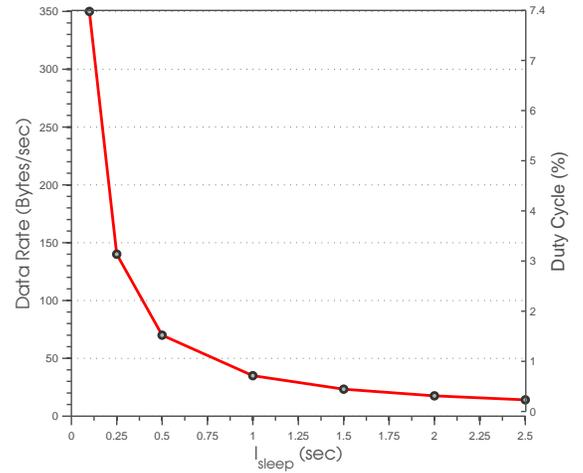
Fig. 9. LAMP Application throughput: varying  $I_{sleep}$  and its duty cycle.
