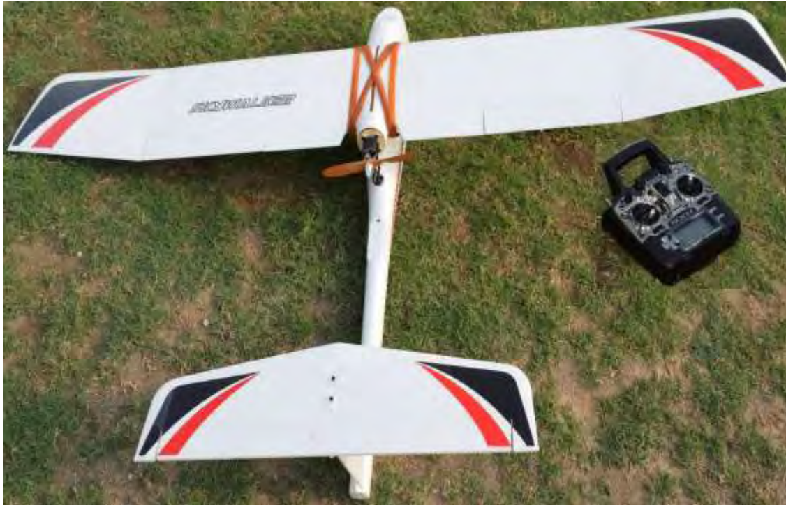
Left figure, developed fixed wing UAV for forestry/agriculture land aerial survey. Right figure, ground control station
